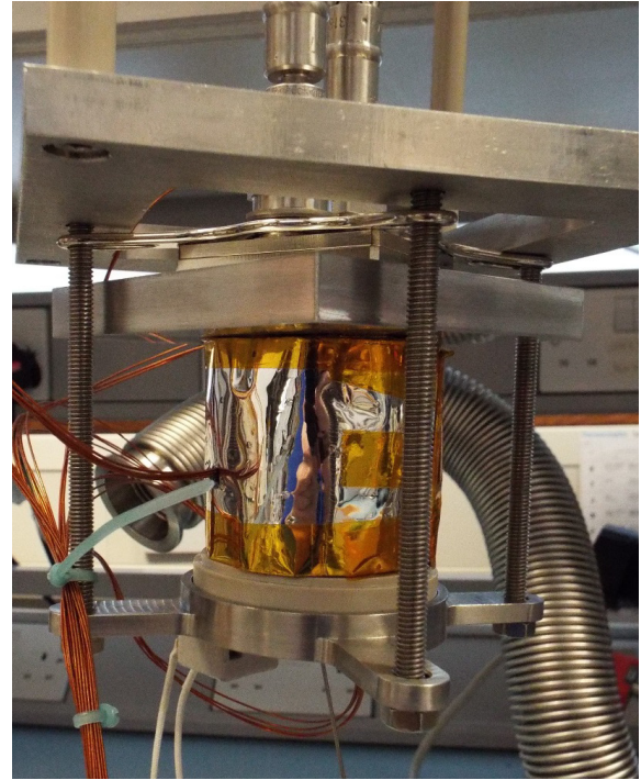
Figure 13: RHU surrounded by MLI, to model the 'mainly conduction' case
