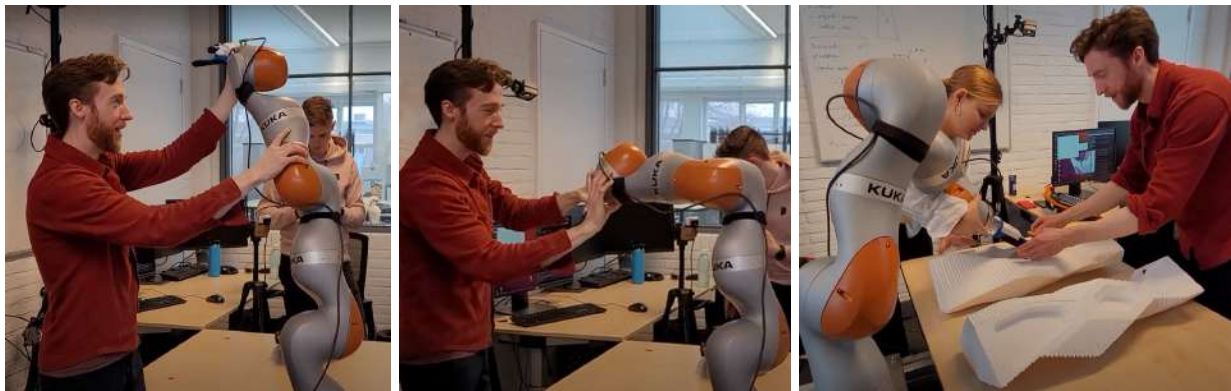
Left to Right: Point A, B, C (Table) in the calibration of the arm
